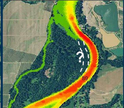
Lack of disturbance transformed former bare gravel bar to mature floodplain. Preliminary modeled inundation and velocity at 40,000 cfs by James White, USGS
