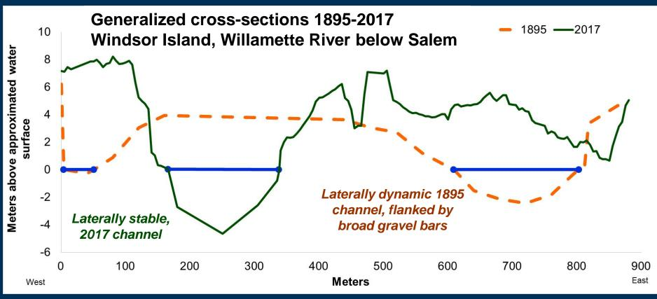
2017 topography from provisional topo-bathy lidar by QSI, Inc. and USGS boat-based surveys; 1895 topography from USACE navigational charts. Provisional data and analyses, subject to revision. Prepared by Gabe Gordon, USGS.
